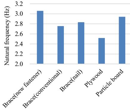
**Figure 4:** Natural frequency of shear walls
