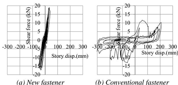
Figure 8: Shear force-story displacement relationship under JMA Kobe 100% input
