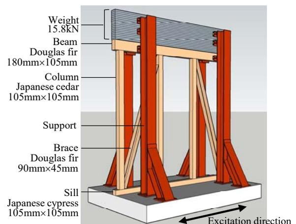
Figure 2: Test apparatus and specimen
