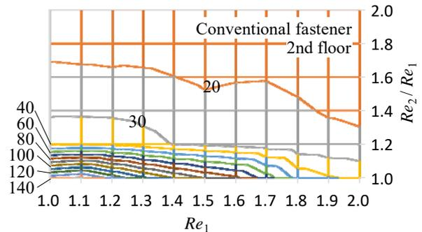
Figure 18: Maximum story displacement of braced shear wall with conventional fastener (unit: mm)
