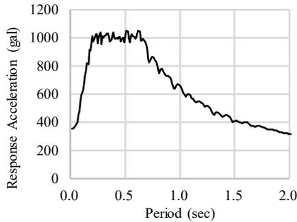
Figure 15: Response acceleration spectra of BCJ L2 wave ( $h=5\%$ )
