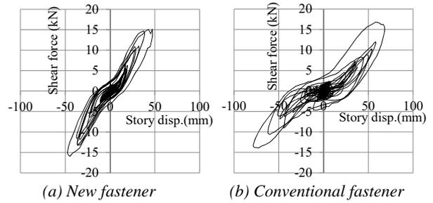
Figure 9: Shear force-story displacement relationship under Mashiki 70% input
