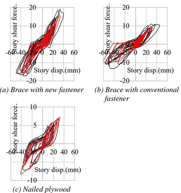
Figure 14: Hysteresis models of shear walls (black line: shake table test, red line: model)
