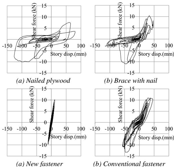
Figure 7: Shear force-story displacement relationship under JMA Kobe 60% input
