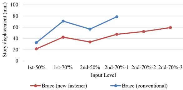
Figure 11: Maximum displacement under Mashiki input
