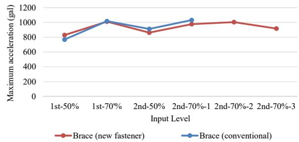
Figure 13: Maximum response acceleration under Mashiki input
