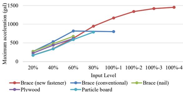
Figure 12: Maximum response acceleration under JMA Kobe input
