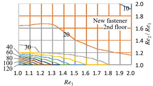
Figure 17: Maximum story displacement of braced shear wall with new fastener (unit: mm)
