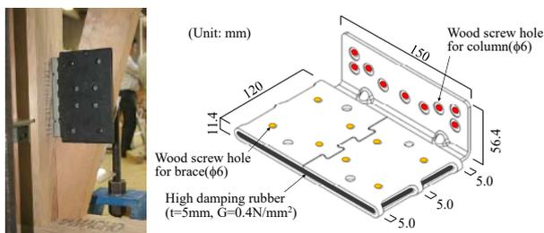
Figure 1: New developed brace fastener
