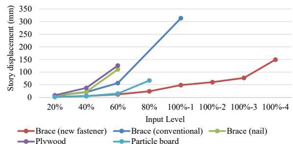
Figure 10: Maximum displacement under JMA Kobe input
