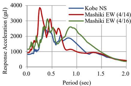
**Figure 3:** Response acceleration spectra
