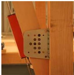
Picture 2: New brace fastener installed at the end of brace
