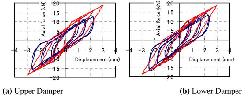
**Figure 4.2.** Non-linear Hysteresis Models of Dampers for K-braces
