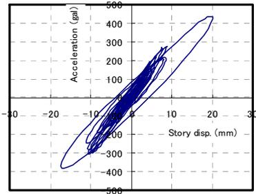
Figure 5.4. Measured Acceleration - Story displacement Relationship of the Frame with K-braced Dampers under Shaking Table Test
