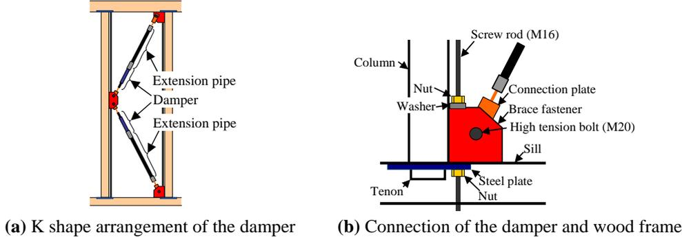
Figure 2.3. Installation of damper and its connection
