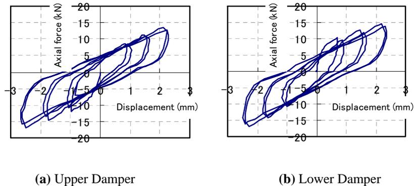
**Figure 5.2.** Force - Displacement Relationship of K-braced Dampers under Quasi-static Loading Test
