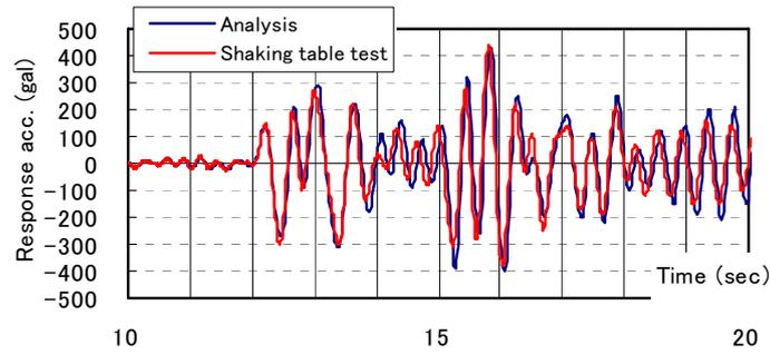
**Figure 5.6.** Response Accelerations of the Frame with K-braced Dampers by Analysis and Shaking Table Test (JMA Kobe NS)
