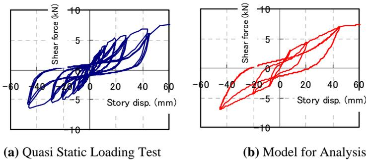
**Figure 4.3.** Force-Displacement Relationships and Non-linear Hysteresis Models of Nailed Plywood Panels
