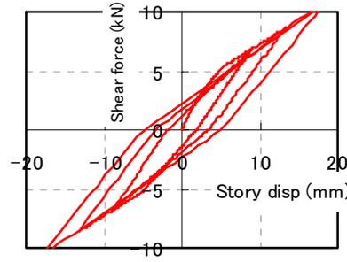
**Figure 4.5.** Non-linear Hysteresis Model of the Frame with K-braced Dampers by Push Over Analysis
