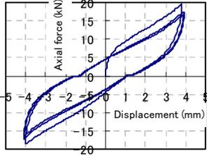
**Figure 2.2.** Force-Displacement Relationships of a Damper using High Damping Rubber
