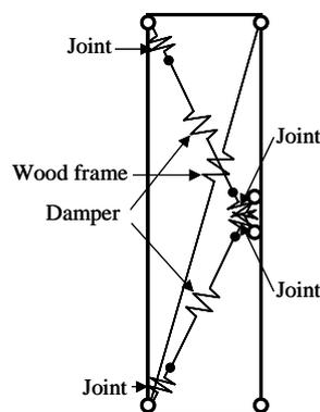
**Figure 4.1.** Schematic Models of Frame with Dampers for Response Analysis
