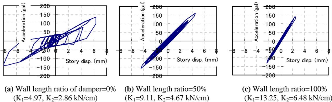
**Figure 5.7.** Response of the Frame with Dampers and Nailed Plywood Shear Panels under JMA Kobe Motion ( $W=22.295$ kN, Input=70.98gal)
