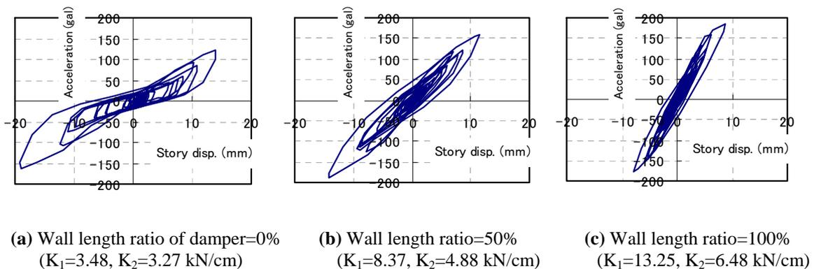
**Figure 5.8.** Response of the Frame with Dampers and Double Wood Braces under JMA Kobe Motion ( $W=35.672$ kN, Input=93.34gal)
