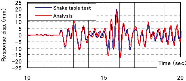
Figure 5.5. Response Displacements of the Frame with K-braced Dampers by Analysis and Shaking Table Test (JMA Kobe NS)
