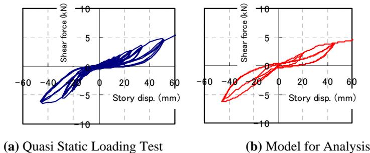
**Figure 4.4.** Force-Displacement Relationships and Non-linear Hysteresis Models of Single Wood Braces
