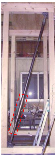
Picture 2. Setup of the damper device
