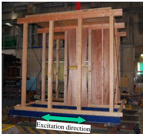
Picture 4. Wood frame specimen for shaking table test
