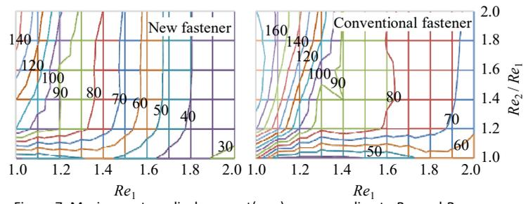
Figure 7: Maximum story displacement (mm) corresponding to  $Re_1$  and  $Re_2/Re_1$
