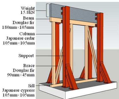
Figure 2: Test apparatus and specimen
