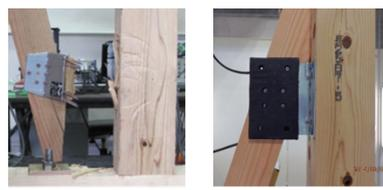
(a) Conventional fastener (b) New fastener
