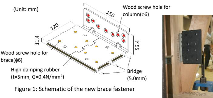
Though maximum story displacement of the braced wall with conventional brace fasteners was over 300mm, the one with the new brace fasteners was approximately 50mm under 100% of JAM Kobe wave. After following three 100% JMA Kobe waves were input to the specimen, the maximum displacement increased to 150mm.
